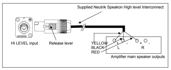
High Level connections should be made to the same binding posts as the main speakers. Connect as shown above. Red to the amplifier's primary right speaker red terminal, yellow to the amplifier's primary left speaker red terminal and black to one of amplifier's primary speaker black terminals (not both).
